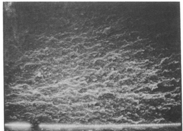
Figure 14 Tear fractograph of 30 phr HDPE filled NR vulcanizate aged for 1 day at 100°C (100×).
